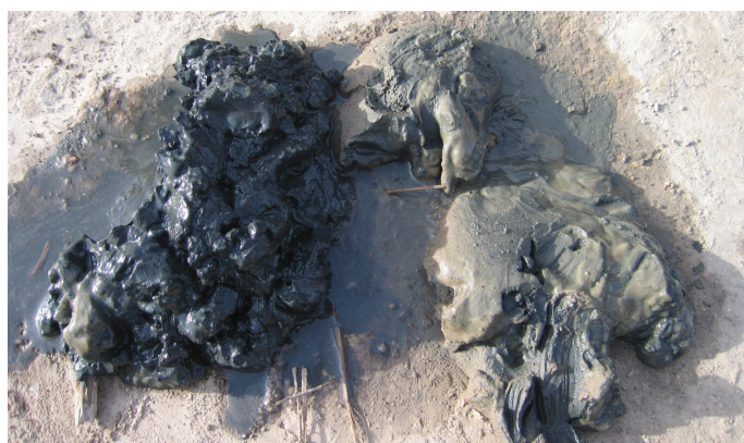
Fig. 1. On the left is a bottom soil sample from a pond suffering from the effects of hydrogen sulfide. Note the black color. On the right is a sample from a healthy pond. Note the normal soil color.
