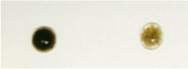
Fig. 5. Treated settled sludge samples from the bottom of a lagoon (left) appear darker than untreated settled sludge (right). The dark color of the treated settled sludge shows that it is further oxidized, which is an indication of increased biological activity compared to untreated areas.
