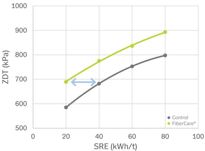
**Fig. 3 Comparison of refining energy use**
