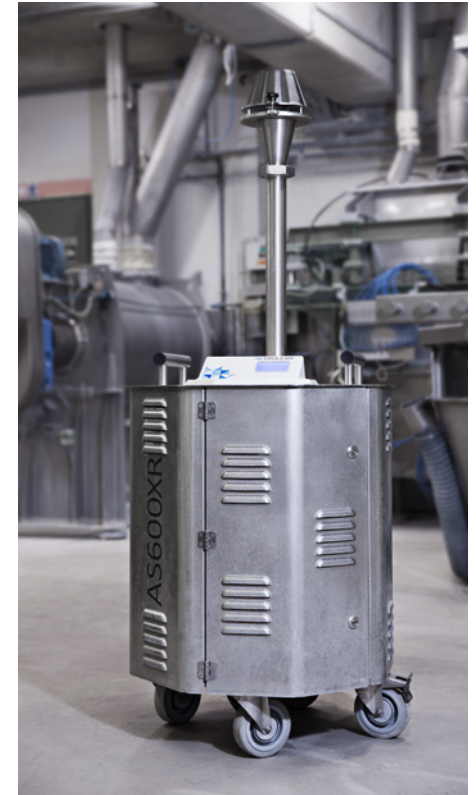
Stationary high-volume pump Used for measurement of area exposure
